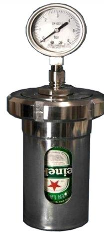
Suitable tool for measuring the pressure and therefore the CO<sub>2</sub> content existing in metal cans (beer, coca cola, sprite, etc.). The can of pyrometer can measure the pressure inside an aluminum can quickly and with high precision.
